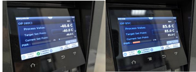
Figure 25 - Environmental chamber control panel at temperature extremes
