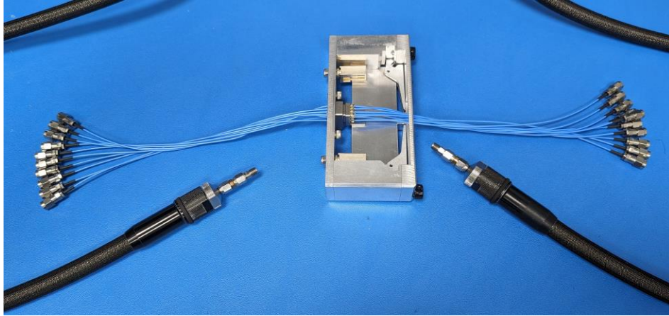
Figure 8 – VSWR & Insertion Loss Test Set Up, Test Group 5 & 6 shown
