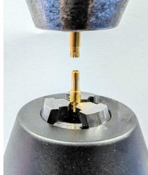
Figure 6 - Test Groups 1 and 2 mounted for mating force testing
