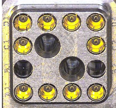
Figure 15 – Test Groups 1 and 2 mounted in the CheckMate durability tester
