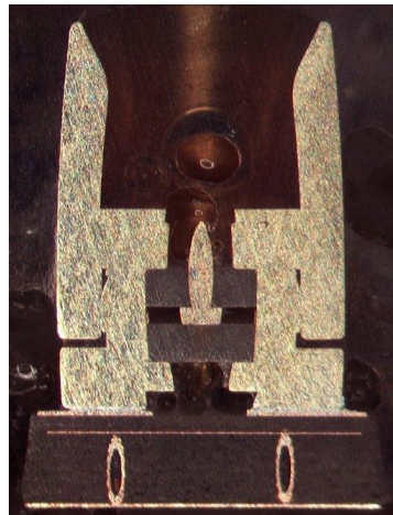
Figure 8: Cross-Section of SK-3400 (PEEK)
