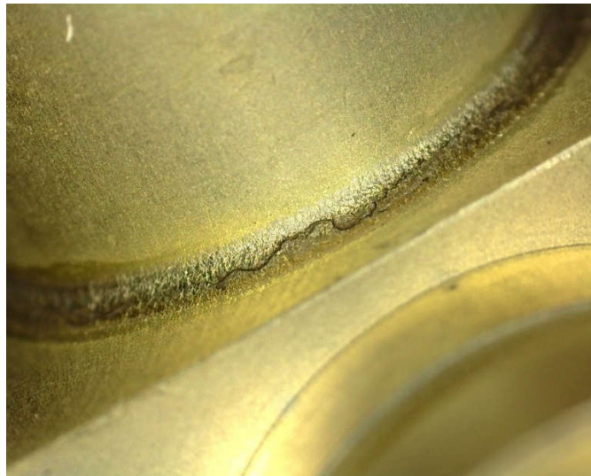
Cracked brazed joint
