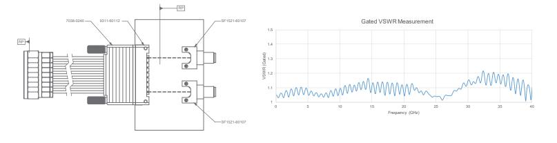
Gated VSWR measurement in above image consists of Mini-D RF cable assembly (7038-0240) and mating connector (9311-60112) plus ~.25" PCB after launch transition.
