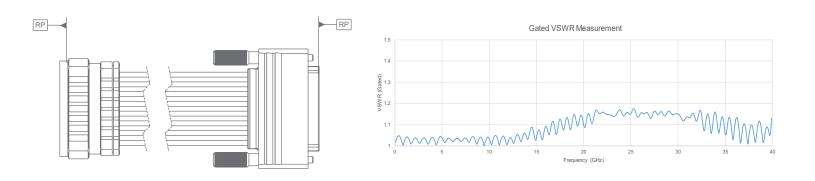
Gated VSWR measurement in above image consists of discrete 6" Mini-D RF cable.
