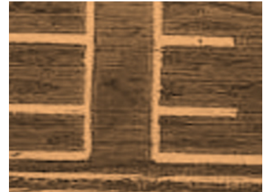
Filled Blind Microvia
