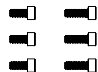
18-8 STAINLESS STEEL 2-56 MOUNTING SCREWS QTY: 3X .188" LONG, 3X .250" LONG
