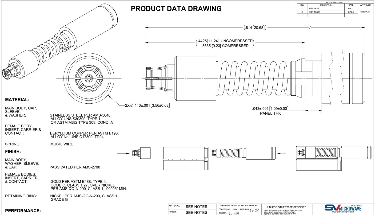
IMPEDANCE: 50 OHMS FREQ. RANGE: DC TO 40.0 GHz
