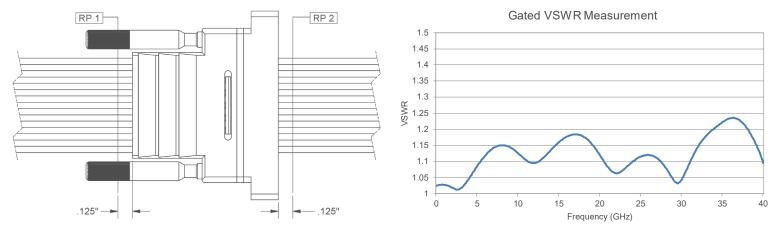
Gated VSWR measurement was generated using time domain gating at RP1 and RP2 as shown in the above image. Above image consists of Mini-D RF Cable assembly mated to Panel Mount Mini-D RF male cable connector. Cable assemblies terminated to 2.92 mm cable connectors.
