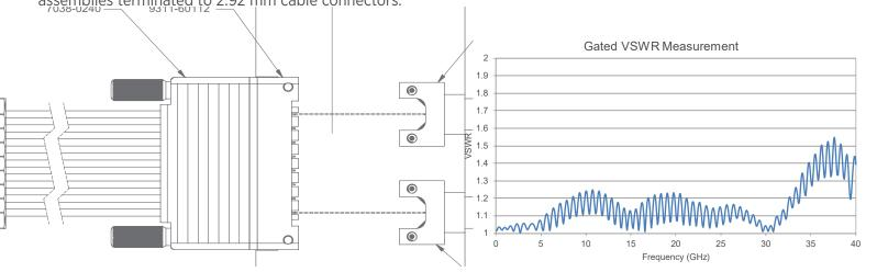
Gated VSWR measurement in above image consists of Mini-D RF cable assembly (7038-0211) and mating connector (9311-60112) plus ~.25" PCB after launch transition.
