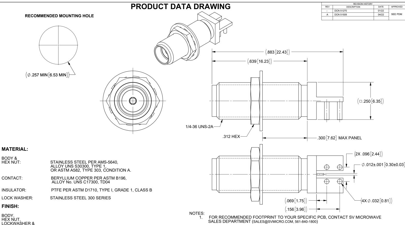
GOLD PER ASTM B488, TYPE II, CONTACT: CODE C, CLASS .76, OVER NICKEL PER AMS-QQ-N-290, CLASS 1, .00005" MIN.
