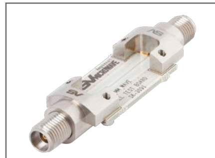
Board level products evaluated for maximum performance through the PCB launch
